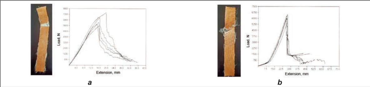
Fig. 9. Maximum breaking force by strip specimen method and corresponding stress-elongation diagrams for fabric 80% p-aramid / 20% PES: a – testing in the warp direction (U); b – testing in the weft direction (B)
